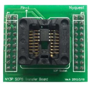
Flip over the board and short-circuit SOP Socket Pin-1 and Pin-4 as the picture below:
